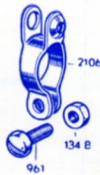
(Code No. 52/2), Ref. 2112. CABLE (O/Casing) STOP, fits on Rear Chain- stay.
