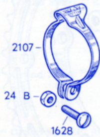
(Code No. 52/1), Ref. 2111. CLIP for Outer Casing, fits Frame Tube 1 1/8" D.
