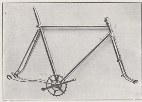
The Brilliant has been designed solely for the racing man, a semi upright model allowing full scope for position and fitted with our Rear Vibrant Triangle (patent No. 33317) The vibratory action caused when riding over uneven ground lessens the retarding force on rear wheel, resulting in less loss of speed.
